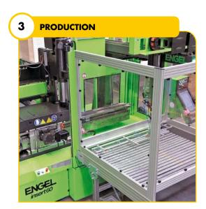
Our automated, state-of-the-art injection moulding production line forms the basis for manufacturing optical componentry. Most photometric optics are produced using either poly(methyl) methacrylate (PMWA) or polycarbonate (PC). These top-quality materials also demand flawless processing.
